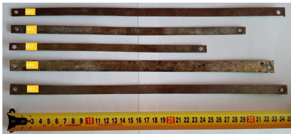
Fig. 2. Experimental samples of plates made of Cu-Al-Mn alloy.
