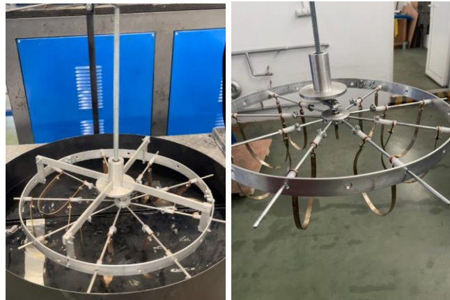
Fig. 8. General view of a heat engine with thermosensitive elements made of Cu-Al-Mn shape memory alloy
