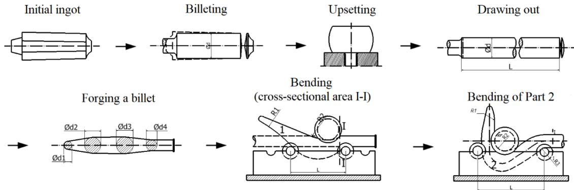
**Fig. 1. Hook forging technology scheme.**
