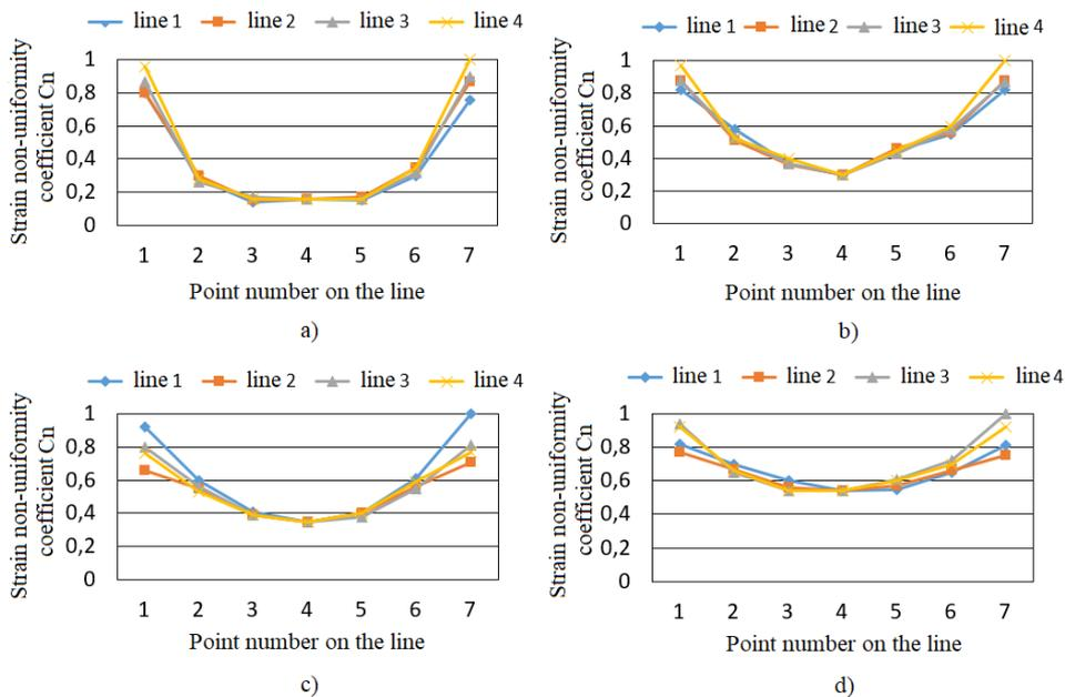
**Fig. 9. Graphs of the distribution of the deformation non-uniformity coefficient during drawing out of billets after the third pass:  $h/D = 1, \epsilon=10\%$  (a);  $h/D = 2, \epsilon=10\%$  (b);  $h/D=1, \epsilon=20\%$  (c);  $h/D=2, \epsilon=20\%$  (d).**
