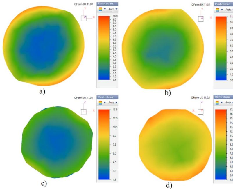
**Fig. 8. Distribution of plastic deformation in the cross-section during drawing out of billets after the third pass:  $h/D = 1, \epsilon=10\%$  (a);  $h/D = 2, \epsilon=10\%$  (b);  $h/D=1, \epsilon=20\%$  (c);  $h/D=2, \epsilon=20\%$  (d).**
