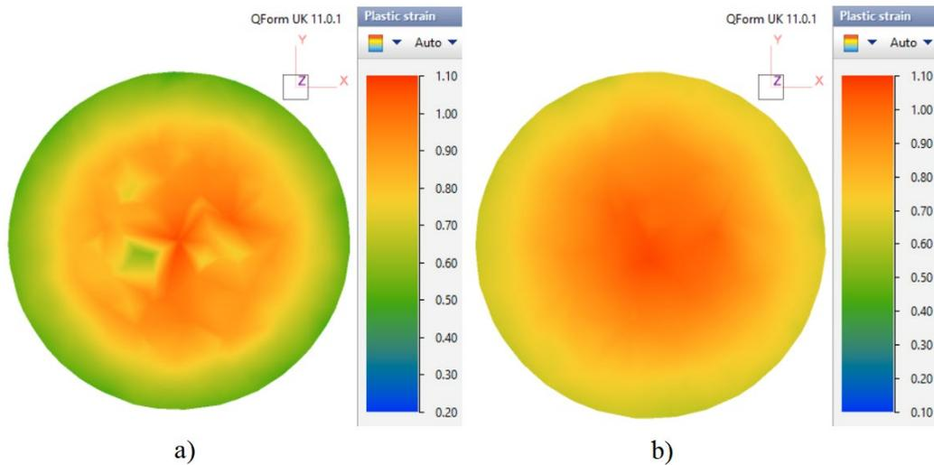
**Fig. 6. Distribution of plastic deformation in the cross-section during billet upsetting: shape factor  $h/D = 1$ , strain  $\epsilon = 50\%$  (a); shape factor  $h/D = 2$ , strain  $\epsilon = 50\%$  (b).**
