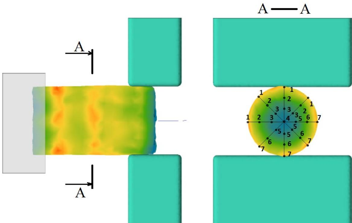
Fig. 5. Schematic arrangement of lines and control points in the cross-section of the billet during the drawing-out process.
