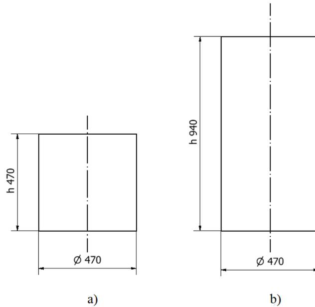
**Fig. 2. Sketches of initial billets for upsetting with shape factors:  $h/D = 1$  (a) and  $h/D = 2$  (b)**
