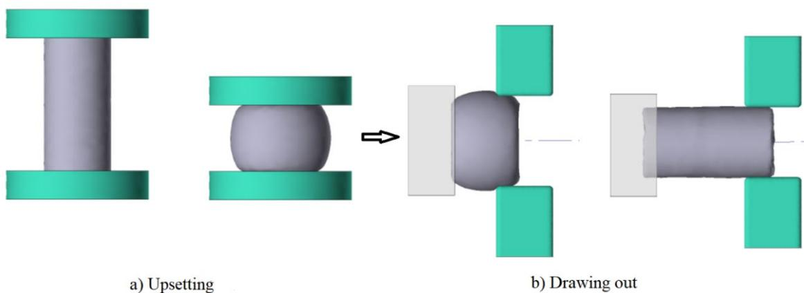
**Fig. 3. 3D model of the upsetting process (a) followed by the drawing-out process (b).**
