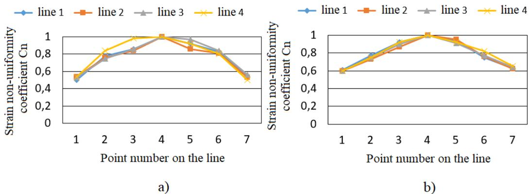
**Fig. 7. Graphs showing the distribution of the deformation non-uniformity coefficient during billet upsetting: shape factor  $h/D = 1$  (a), and  $h/D = 2$  (b).**
