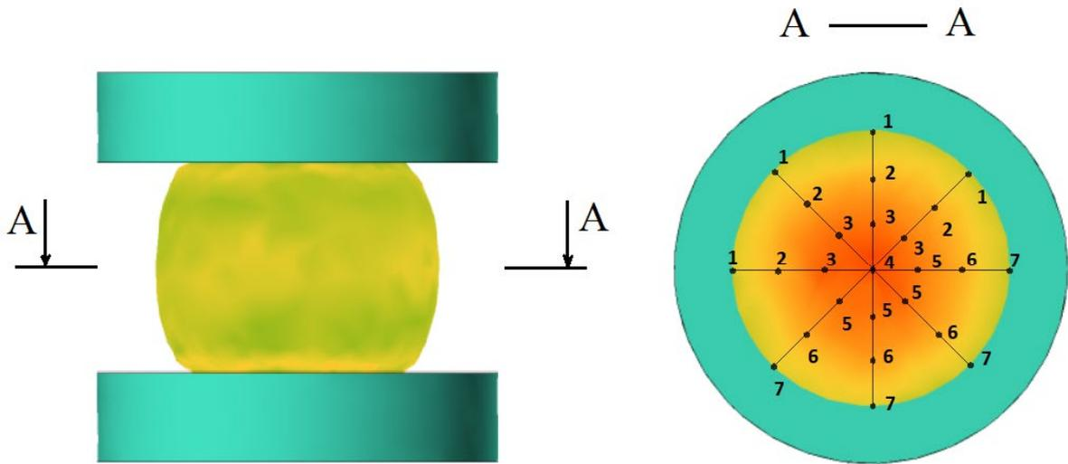
Fig. 4. Schematic representation of lines and control points in the cross-section of the billet during the upsetting process.
