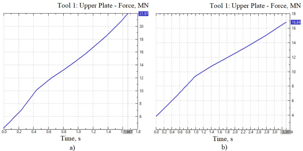
Fig. 10. Graphs of the deformation force versus time for two upsetting processes: (a)  $h/D=1$  and (b)  $h/D=2$  ( $\epsilon=50\%$ ).
