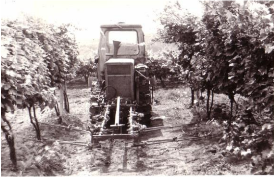
Figure 1.3. Tractor unit with automatic guidance system (AGS) using stems of grapes.
