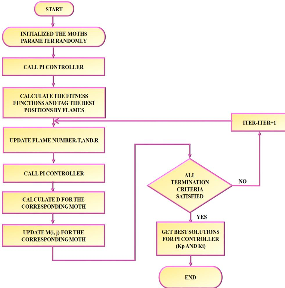
Fig. 4. Flowchart of MF optimized PI controller.
