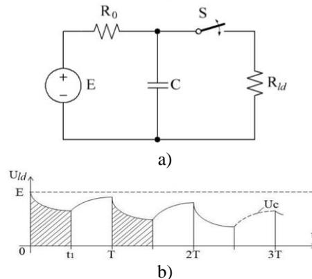
Fig. 2. Impulse operation mode of a source.
