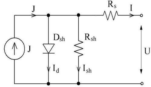
Fig. 5. Solar battery equivalent circuit.
