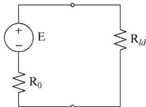
Fig. 1. Source to load connection circuit.
