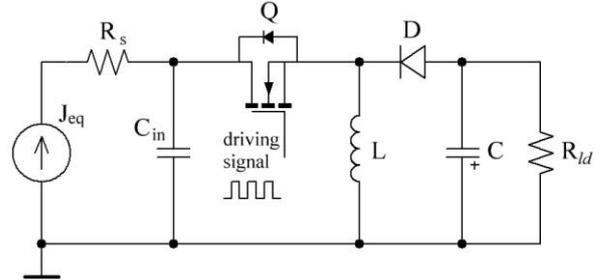
Fig. 7. The circuit with input equivalent current source.
