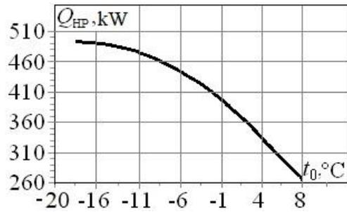
$t_{HP}$  – heat load of HPI;  $t_0$  – outdoor temperature
