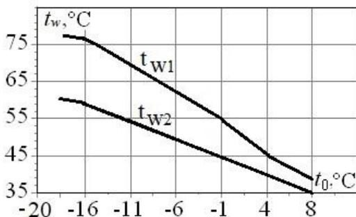
$t_{w1}$  – inlet temperature;  $t_{w2}$  – outlet temperature;
