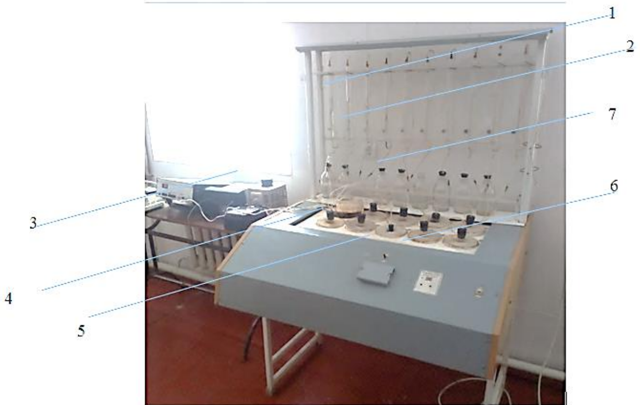
1, 2 – measuring tube of biogas output from bioreactors, 3 – teslameter, 4 – laid stators with a substrate, 5 – the substrate is laid, 6 – a moving platform for mixing the substrate of test samples, 7 – container with lime water.
