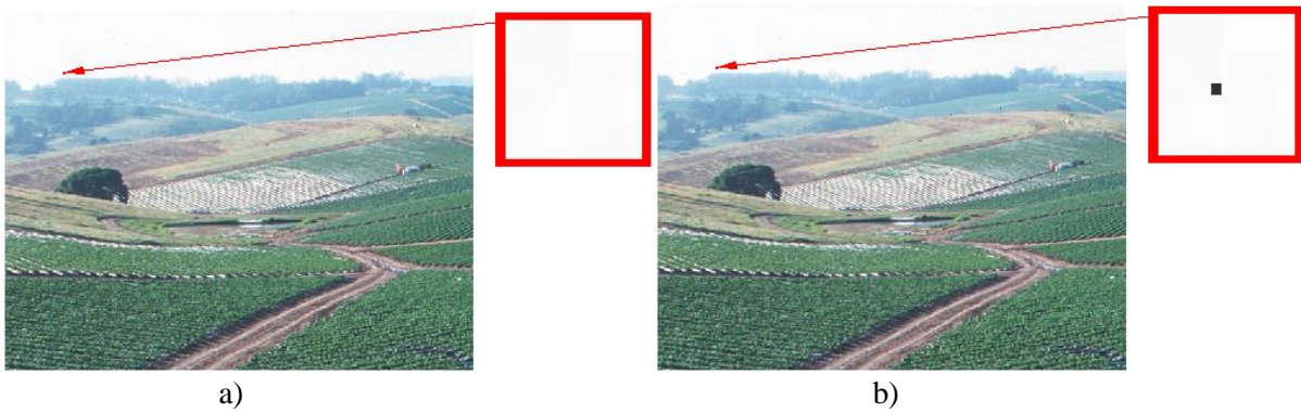
Fig. 7. Local changes of the DI: a) the original image with the selected original 8 \times 8 -area; b) image, the integrity of which is violated within the selected 8 \times 8 -area
