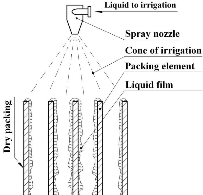
**Figure 2.** Irrigation of the structured packing with spray nozzle
