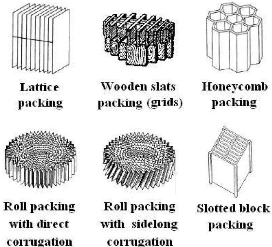
**Figure 1.** *Various structured packings*
