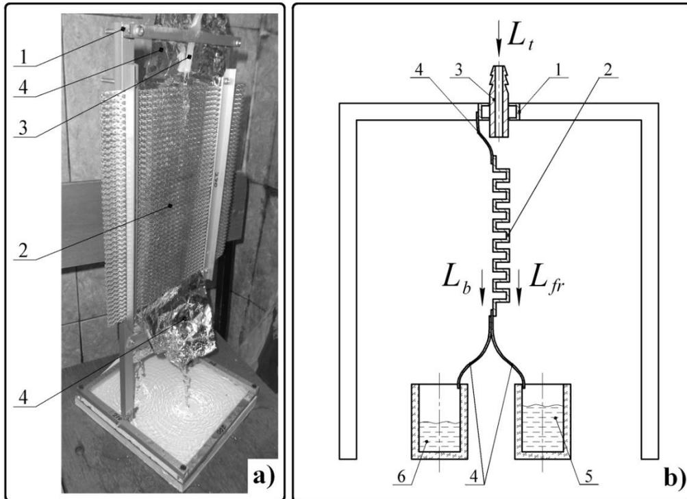
**Figure 6.** Experimental setup a) – isometric view; b) – scheme; 1. base, 2. packing element, 3. inlet jet nozzle, 4. impingement sheets, 5, 6. beakers,  $L_t$  – liquid for irrigation,  $L_{fr}$  – liquid, collected from the front side of the packing element,  $L_b$  – liquid, collected from the back side of the packing element
