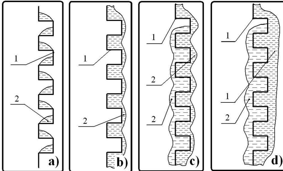
**Figure 7.** Scheme of the liquid flowing on the surface of the packing element in different wetting types: a) flow regime with partial wetting; b) front side flow regime with "standing waves"; c) both sides flow regime with "standing waves" d) flow regime with flooding. 1. element of structured corrugated packing with slits; 2. fluid
