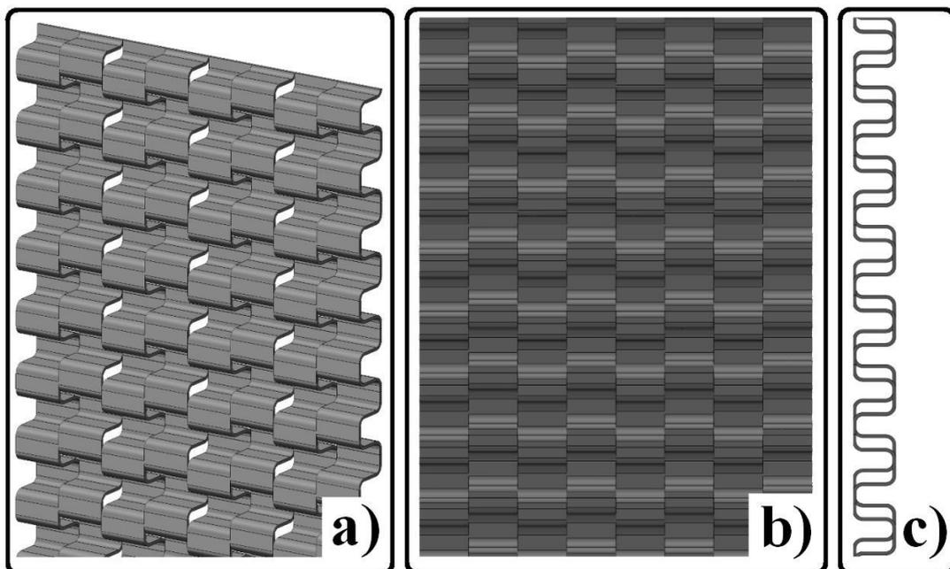
**Figure 4.** Element of the structured corrugated packing with slits, a) – isometric view, b) – front view, c) – side view
