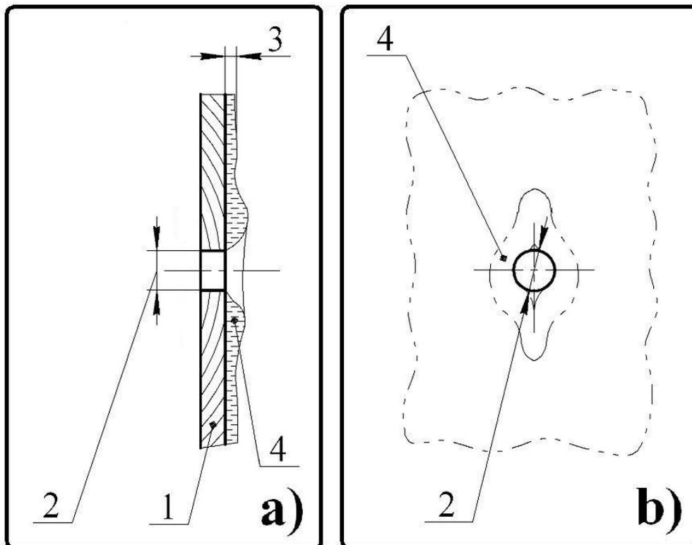
**Figure 3.** Scheme of the falling fluid film around cylindrical hole in the packing, a) – longitudinal section, b) – front view; 1 – element of structured packing, 2 – hole in the packing, 3 – thickness of the fluid film, 4 – local increasing of the fluid film thickness
