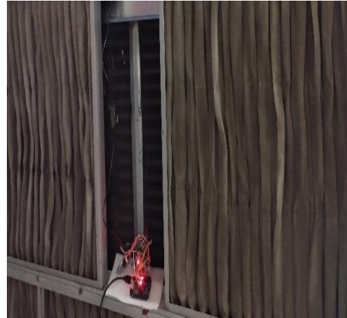
Fig. 1. Data acquisition using an Arduino-based IoT measurement system (i) Hardware setup (ii) Hardware setup for weather data collection (iii) Hardware setup for indoor zone thermal data collection.
