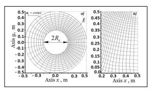
Fig. 4. Electrical field distribution in the hollow cylinder: a) - in the cross-section with the coordinate z = H / 2 = 0.25 m; b) - in the plane of the vertical section - y = 0 and Ra < x < Rb.
