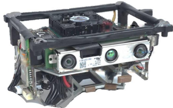
Fig. 2. External view of the hardware of the proposed UAV control system.
