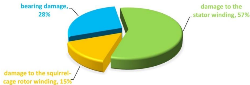
Fig. 1. Damageability of the main elements of an induction motor.
