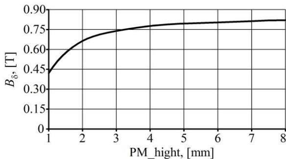
**Fig. 8. Dependence of magnetic flux density in the generator air gap on the PM height.**
