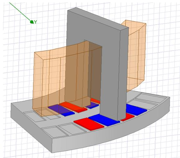
**Fig. 4. 1/8 part of 3D TFM model for analysis.**
