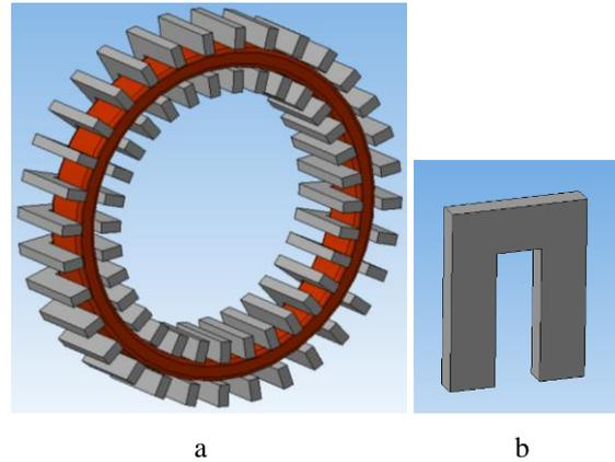
a – one phase of the stator; b – stator pole.
