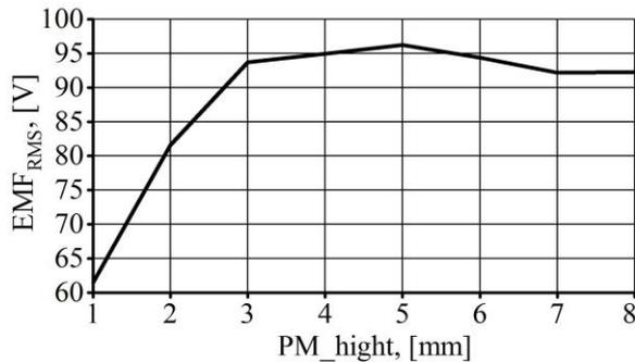
Fig. 5. Dependence of the PMs height on generated EMF value in the stator coil.
