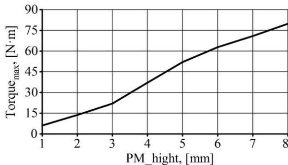
Fig. 6. Dependence of the PMs height on the maximum value of the cogging torque.
