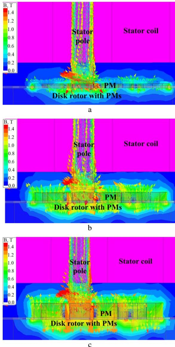
a – PM height 2 mm; b – PM height 5 mm;
