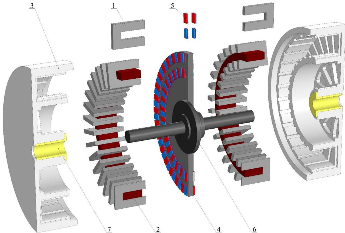
1 – stator pole; 2 – stator coil; 3 – aluminum stator body; 4 – rotor disk made of solid steel;
