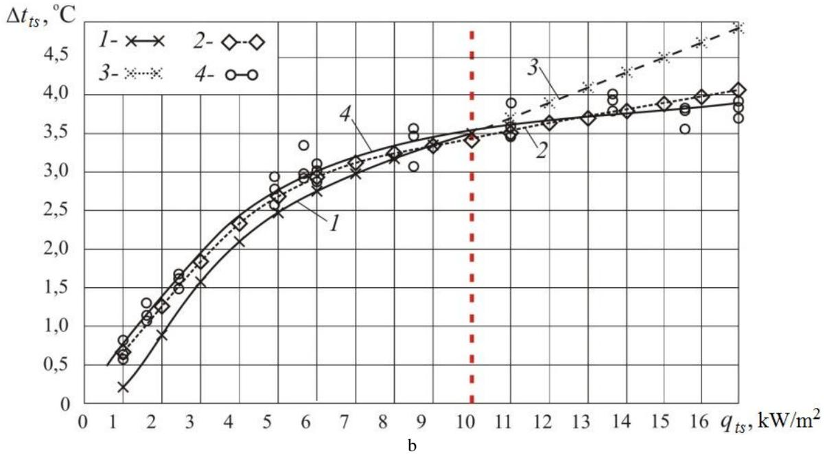
1 - the results of calculations according to the formula (3) at  $q_{ts} < 10 \text{ kW/m}^2$ , 2 - the results of calculations according to the formula (7); 3 - the results of calculations according to the formula (3) at  $10 < q_{ts} < 17 \text{ kW/m}^2$ ; 4 - the experimental results.
