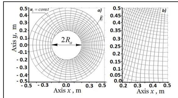
**Fig. 4. Electrical field distribution in the hollow cylinder: a) - in the cross-section with the coordinate  $z = H / 2 = 0.25$  m; b) - in the plane of the vertical section -  $y = 0$  and  $R_a < x < R_b$ .**
