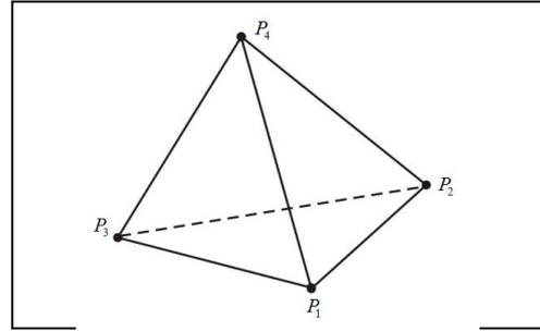
Fig.3. Nodes of tetrahedral from the calculation grid.
